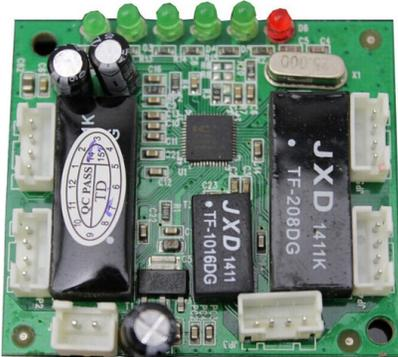
**Figure 6: 5 port OEM Ethernet switch module**
