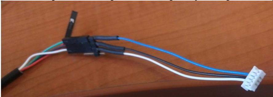
**Figure 1: USB Serial cable wired to 5 pin Picoblade serial connector**
