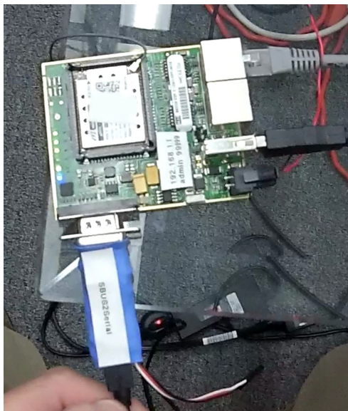
Figure 2: Microhard pDDL motherboard with SBUS2Serial module (USB power taken from Microhard motherboard)
