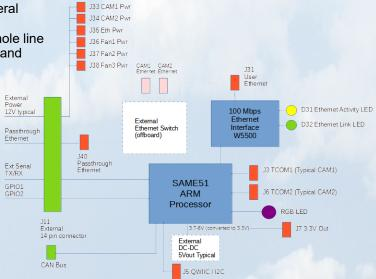
Ethernet Multicomm Board - Block Diagram
