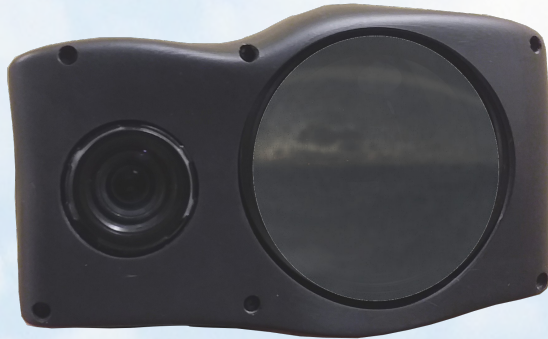
4K+LWIR Continuous zoom on both cameras
